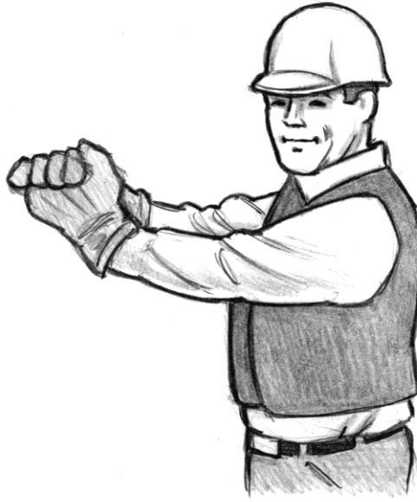
Figure 7-63 – Hold, Dog Drum or Brake Lever (Clasp one hand with the other)
