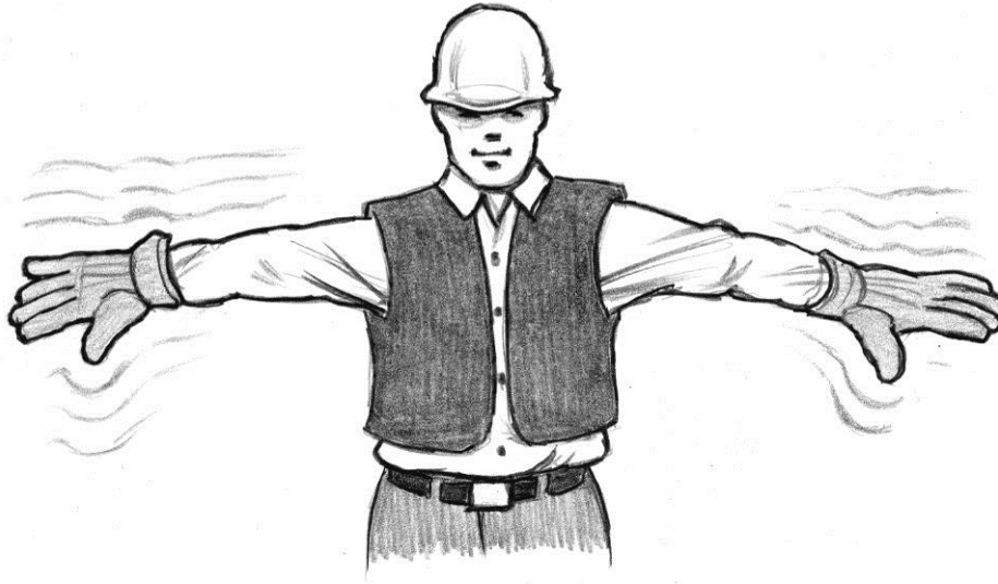
Figure 7-55 – Slack the Mainline Easy (Both hands extended at side, hands fluttering)
