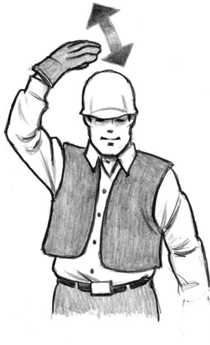
Figure 7-62 – Cable Up (Touch top of head and raise hand up and down)
