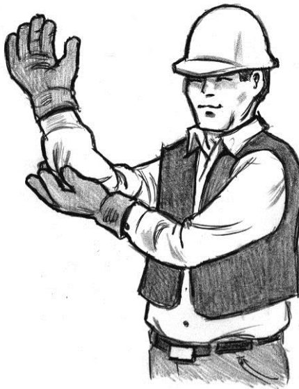
Figure 7-60 – Ahead On The Haywire (Touch hand to bent elbow)
