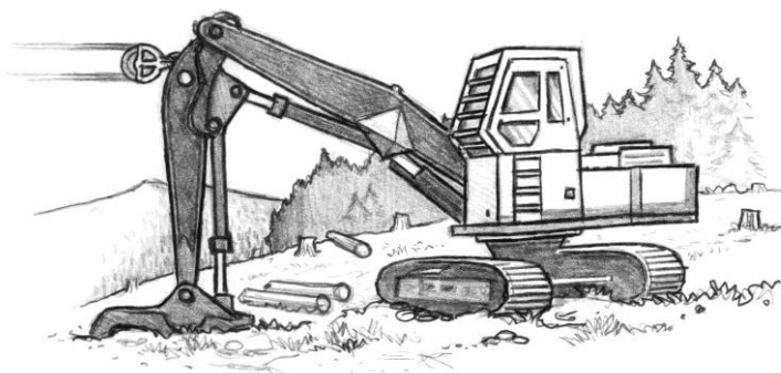
Figure 7-25 – Log Loader Anchor
