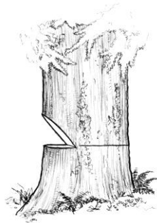
Figure 7-35 – Falling – Conventional Face
