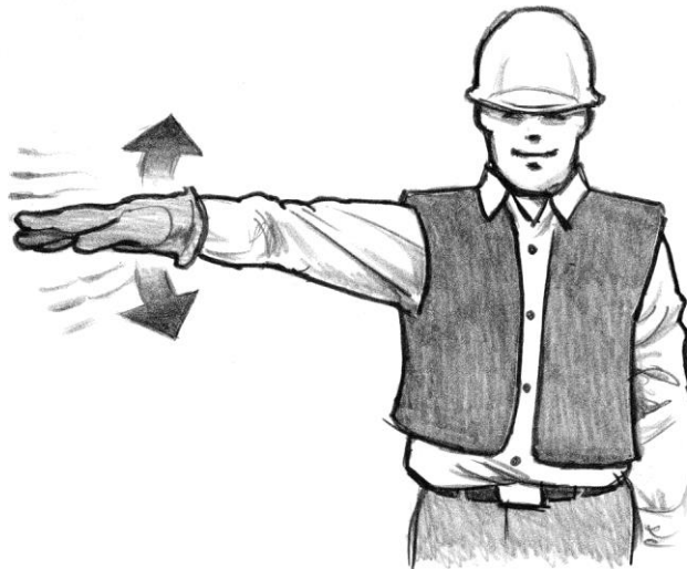
Figure 7-56 – Slack Mainline All Off (Arm extended at side, flipping wrist)
